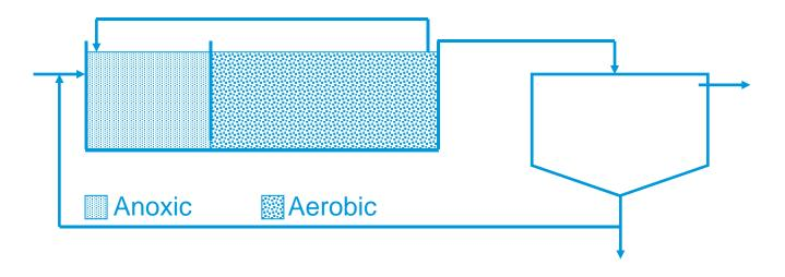
Aerobic zone: DO: 1.5-3mg/L; ORP: +100mV to +350 mV
