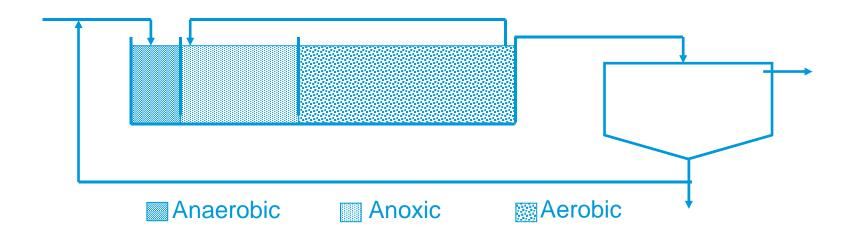
Anaerobic zone: organic phosphates broken down into orthophosphate (release)
