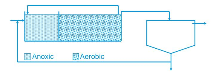
Aerobic zone: ammonia converted to nitrate in the presence of O<sub>2</sub>
